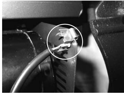
Figure 8.28 Attach grounding clip supplied with the kit to the blower housing. Attach ground wire to grounding clip.
